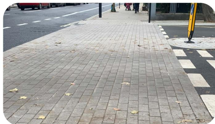
Informal crossing points or continuous pavements would be paved slightly differently from the main pavements, using smaller paving slabs. You can see lots of examples of these around Camden.
