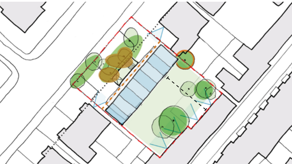
Top: Diagram of the flipped circulation option 1 showing how habitable room to habitable room distances would be under 18m Bottom: Diagram developed as a response to option 1 showing how maintaining the 18m distance required by Camden would push forward the building line along Camden Road and impact the TPO trees.
