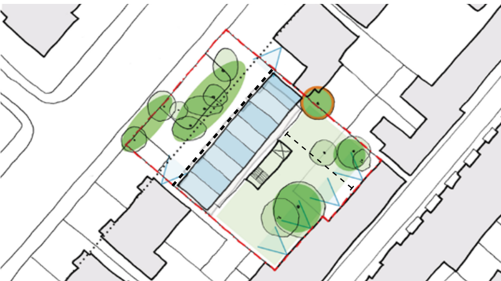
Top: Diagram showing double stacked option 1, the building would be significantly deeper than the existing failing to meet the 18m overlooking distance set by Camden Middle: Alternative to option 1 impacting TPO trees and not achieving the 18m distance for the whole building Bottom: Diagram showing preferred layout
