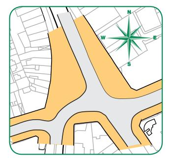
The traffic impact of this option (above) was assessed and would have led to a significant increase in congestion and unacceptable delays to buses and general traffic. Therefore creating a public space on the east side was looked at and found to have a more acceptable impact on traffic with only slightly longer queues than now.
