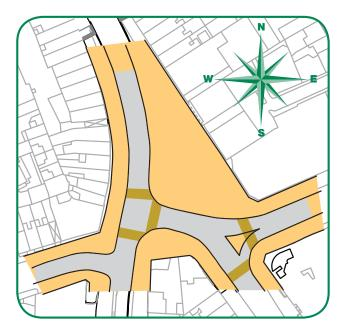
The design concept (left) provided direct and simple pedestrian crossings as well as a safer junction layout for cyclists. These improvements could not be fully achieved with the new public space on the west side.
