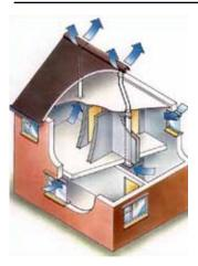
Passive stack ventilation relies on the natural buoyancy of warm air. There are no fans: instead, warm stale air from the bathrooms and kitchen rises through ducts to the ridge of the roof, where it is vented to the outside. Humidity-sensitive trickle vents in the bathrooms and kitchen control the extract rate, and fresh air is supplied by humidity sensitive trickle ventilators in the living area and bedrooms.
