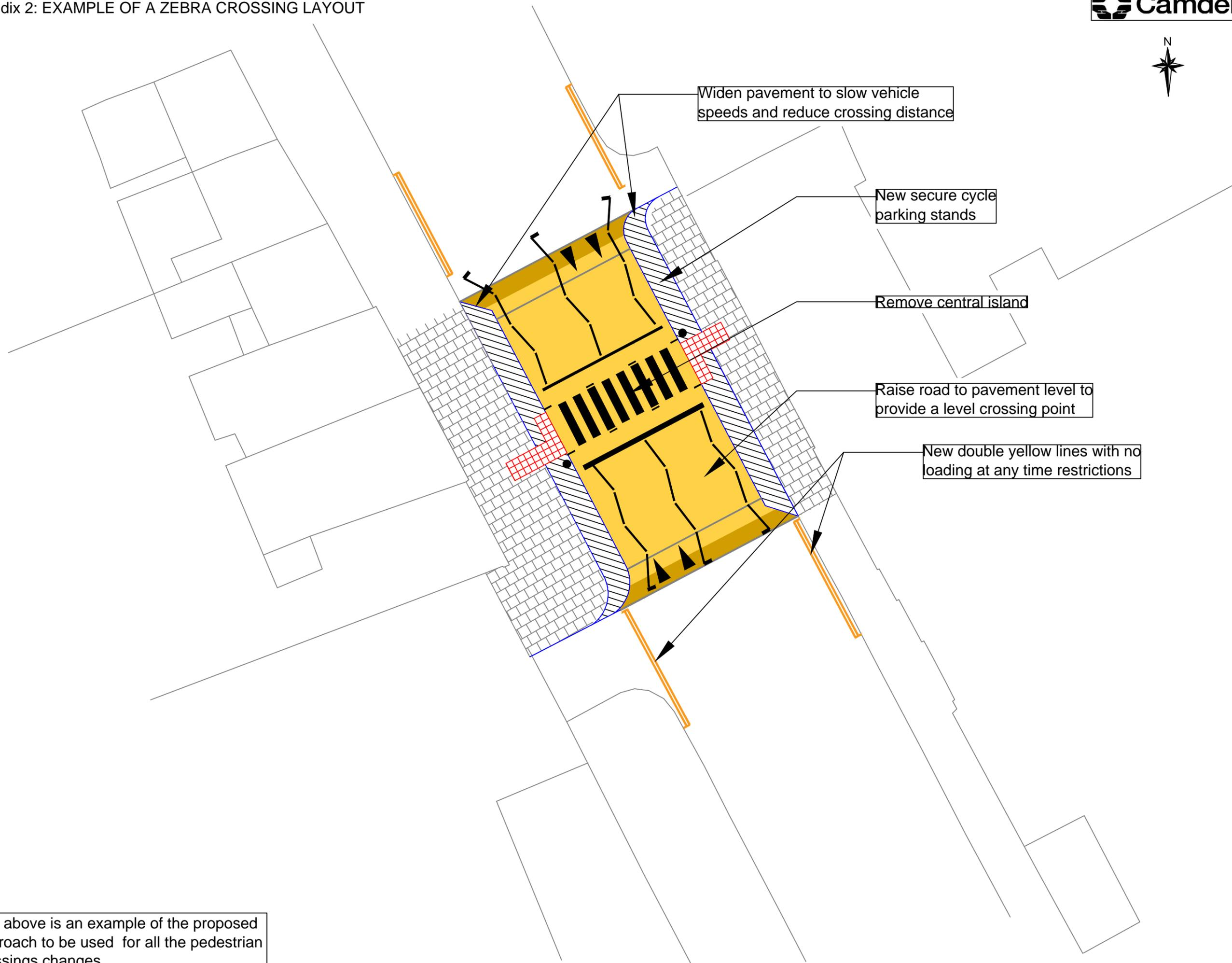
Widen pavement to slow vehicle speeds and reduce crossing distance
