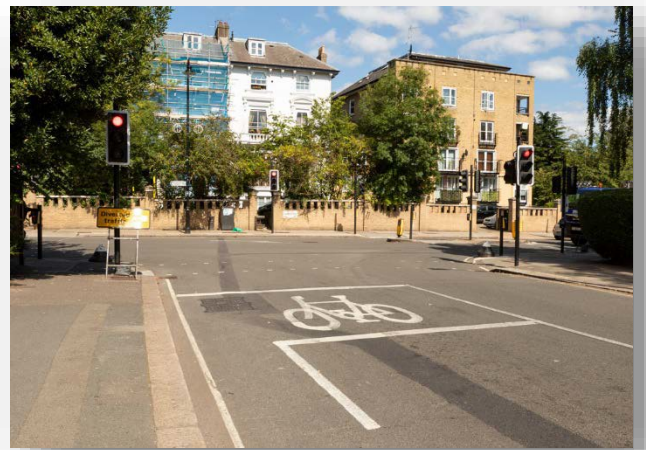
An advanced stop line / cycle box
