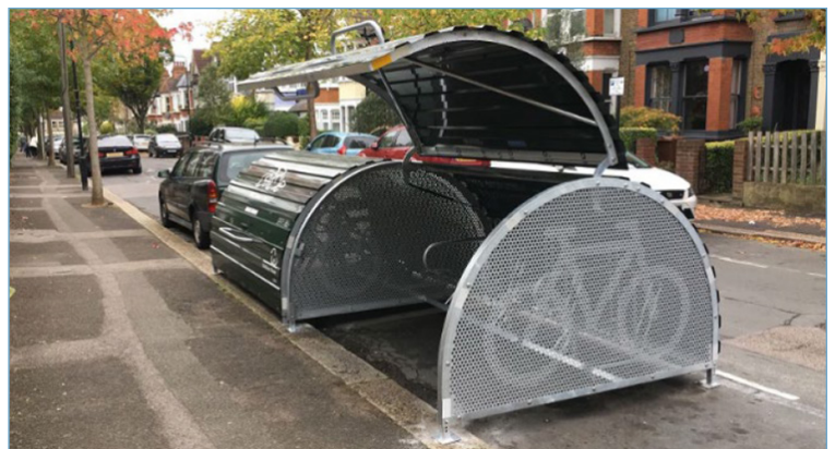
Figure 2: Example of a bike hangar.
