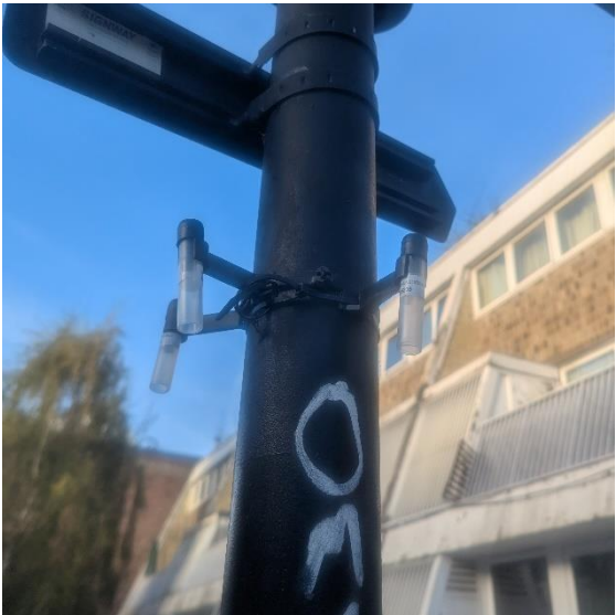
Figure 7 (right): Diffusion tubes for measuring nitrogen dioxide (NO 2 ). There are three tubes here so that we can calculate an average reading, to produce more reliable data.
