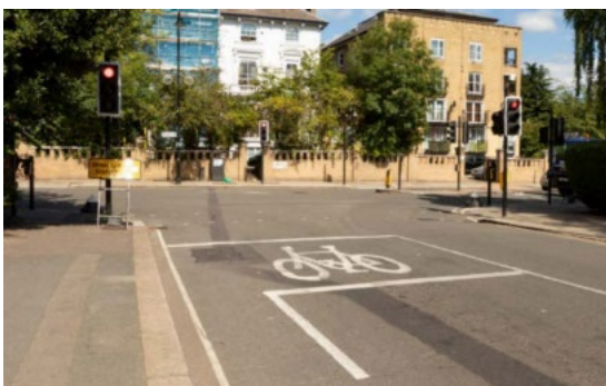
Figure 3.10: Advanced stop line for cyclists
