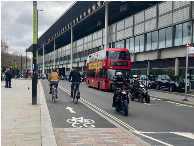
Figure 3.6 Physically separated cycle lanes (this can be done using stepped tracks – as shown in the image, kerbs or wands)
