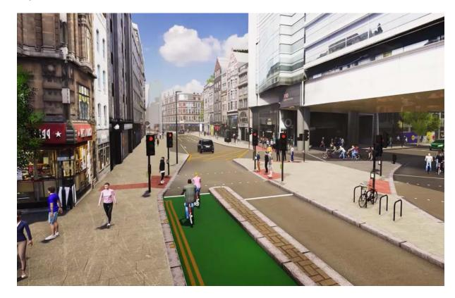
On the High Holborn approach to Southampton Row, a cycle early release would be provided which would allow cyclists to have a 4 second start ahead of motor vehicles to prevent left turning motor vehicles cutting across people cycling. The cycle box would also be increased to 7.5m.
